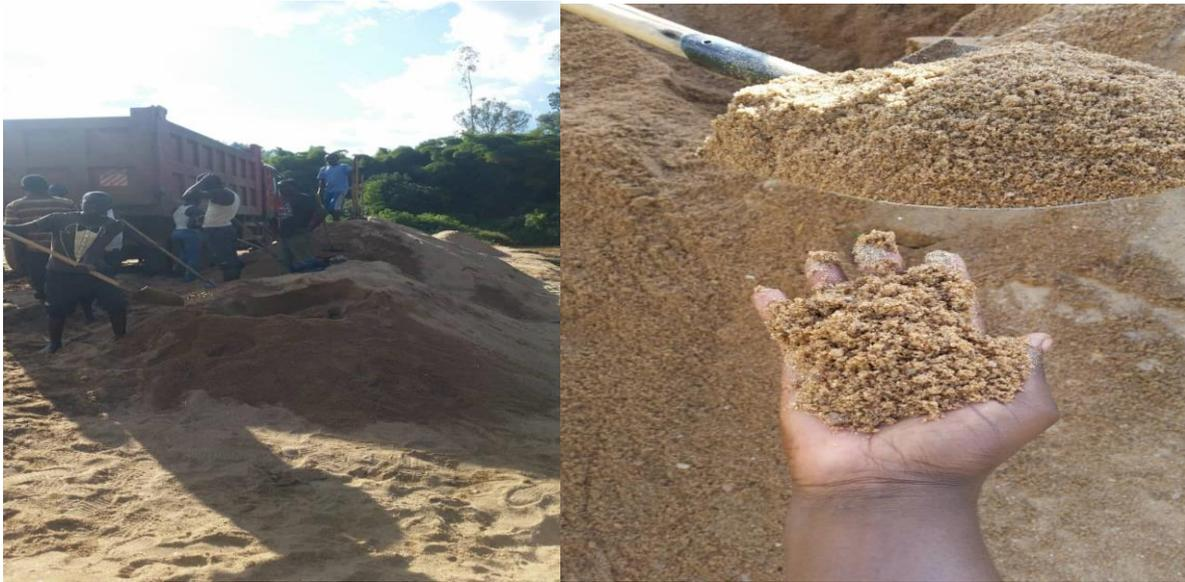
*Sampling Mwogo sand against Mugonero sand to be taken to laboratory for testing in order to decide which sand to use in construction.*
